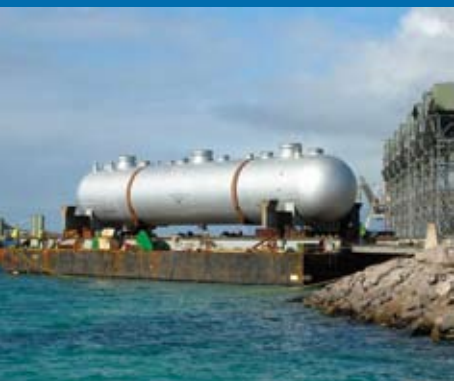
High Pressure Leach Autoclave for the Ravensthorpe Project. It is a six compartment horizontal pressure vessel, constructed of explosion clad titanium. Each compartment is agitated by Titanium agitators.
